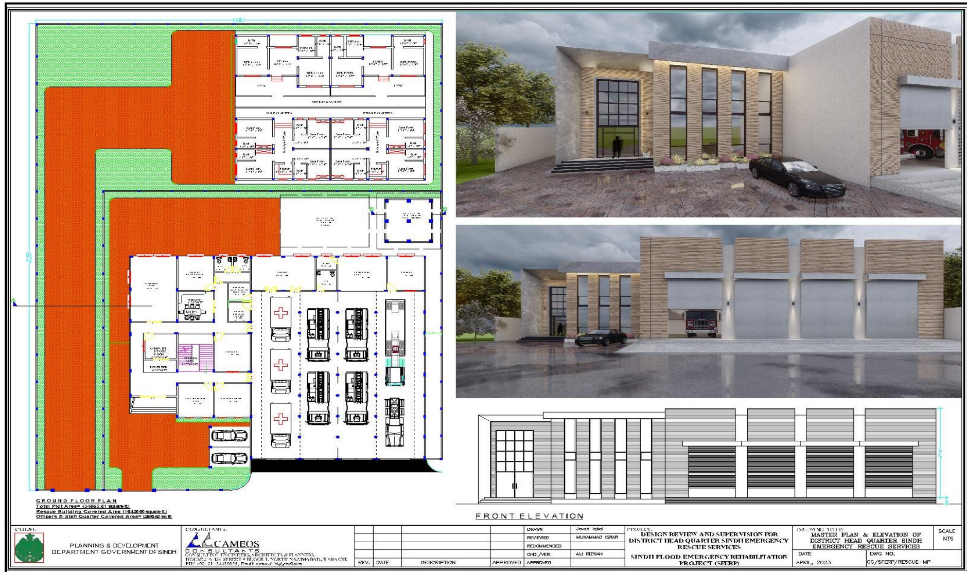
Figure 6: Floor Plan and Front Elevation Drawing of District Level Emergency Rescue 1122 Stations
